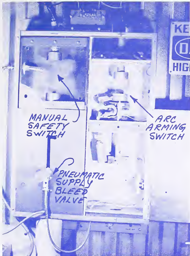
Figure 15—Arc arming switch (ref. fig. 14) (right) and the manual safety switch (ref. fig. 13) (left). Note the pneumatic supply bleed valve just below the switch actuating handle. The high-voltage power supply voltmeter (ref. fig. 17) can just be seen on top of the box containing the switches.
